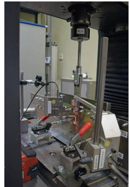
Test set up for shear load testing
