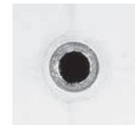
Shiny ring around the bore hole
