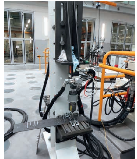
Hilti S-BT HL fastening system under cyclic loading
