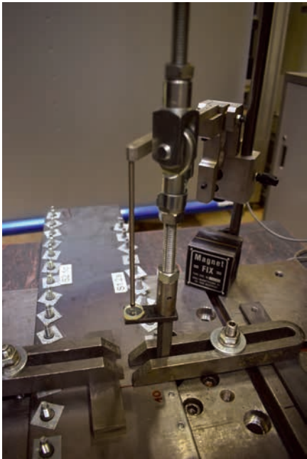
Test set up for tension tests
