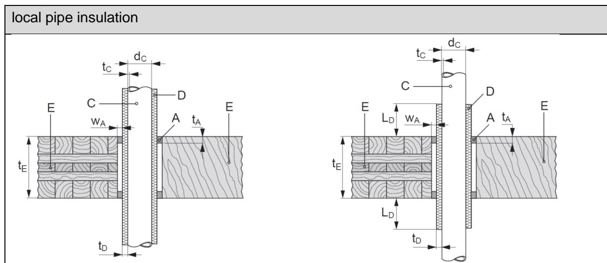
$t_A \geq 25$  mm Hilti Firestop Acrylic Sealant CFS-S ACR (A) on both sides (no backfilling)
