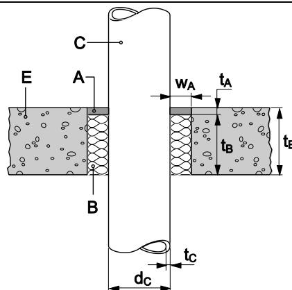
$t_A \geq 15 \text{ mm}$  Hilti Firestop Acrylic Sealant CFS-S ACR (A) on the top side
