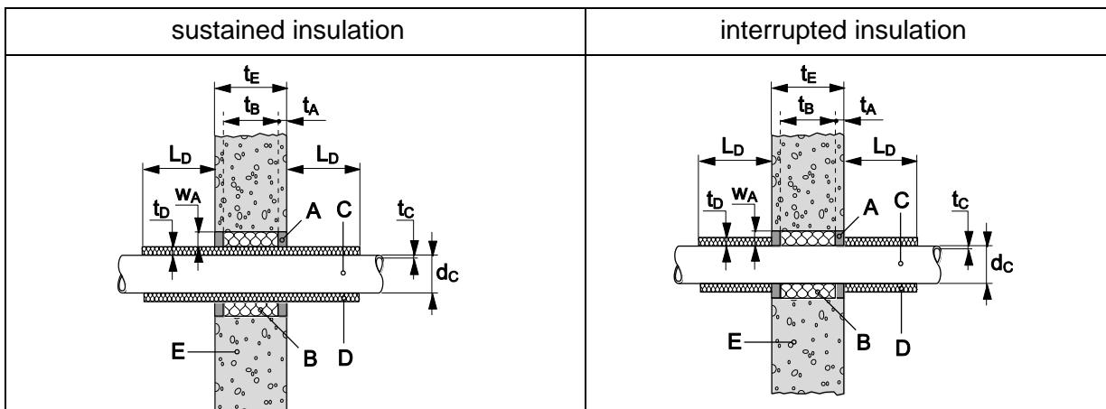
$t_A \geq 20$  mm Hilti Firestop Acrylic Sealant CFS-S ACR (A) on the top side of the floor construction,
