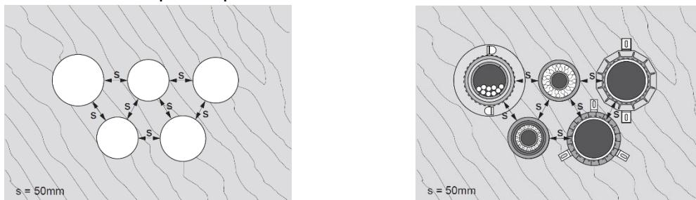
Distances between specific penetration seals - opening to opening (CFS-B, CFS-S ACR, CFS-C EL, CFS-CC):
