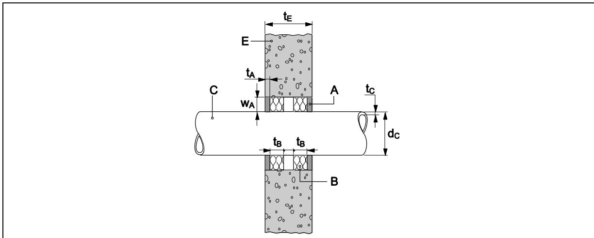
$t_A \geq 15$  mm Hilti Firestop Acrylic Sealant CFS-S ACR (A) on both sides
