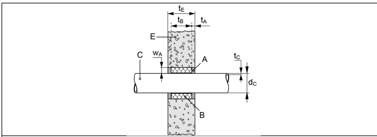
$t_A \geq 15$  mm Hilti Firestop Acrylic Sealant CFS-S ACR (A) on both sides
