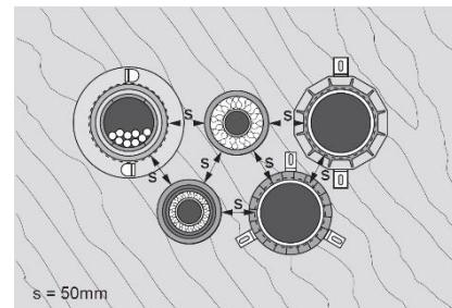
Distances between specific penetration seals - opening to opening (CFS-B, CFS-S ACR, CFS-C EL, CFS-CC):
