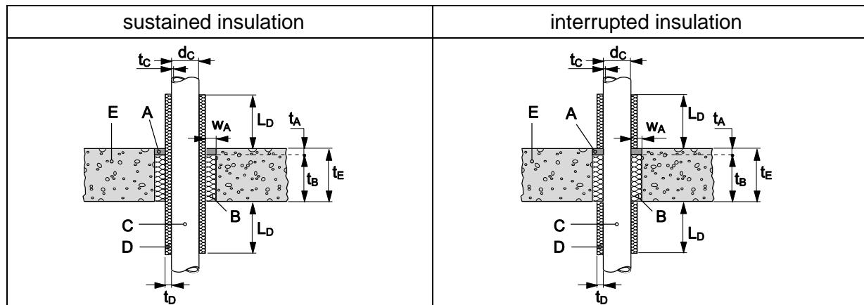
$t_A \geq 10$  mm Hilti Firestop Acrylic Sealant CFS-S ACR (A) on the top side of the floor construction,
