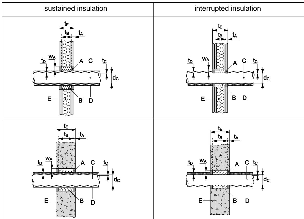
$t_A \geq 10$  mm Hilti Firestop Acrylic Sealant CFS-S ACR (A) on both sides
