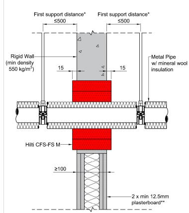
Acoustics rating:  $R_{\text{w}}$  = 50 Maximum opening dimensions: 1200x500mm. For blank openings see approval documents. \*First support and ancillary products should be capable of achieving the same fire performance as the seal and supporting structure.
