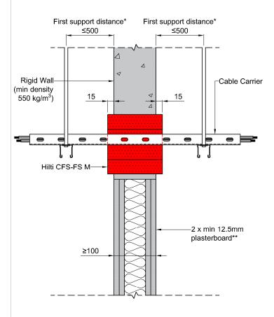
Acoustics rating:  $R_{\text{w}}$  = 50 Maximum opening dimensions: 1200x500mm. For blank openings see approval documents. \*First support and ancillary products should be capable of achieving the same fire performance as the seal and supporting structure.
