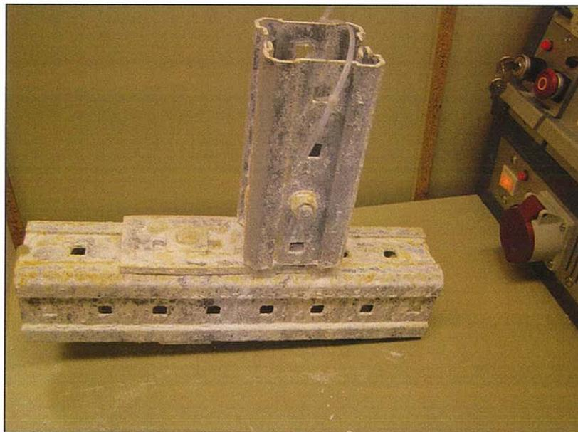
**Pic. 18:** Test object 1 after corrosion resisting conditioning
