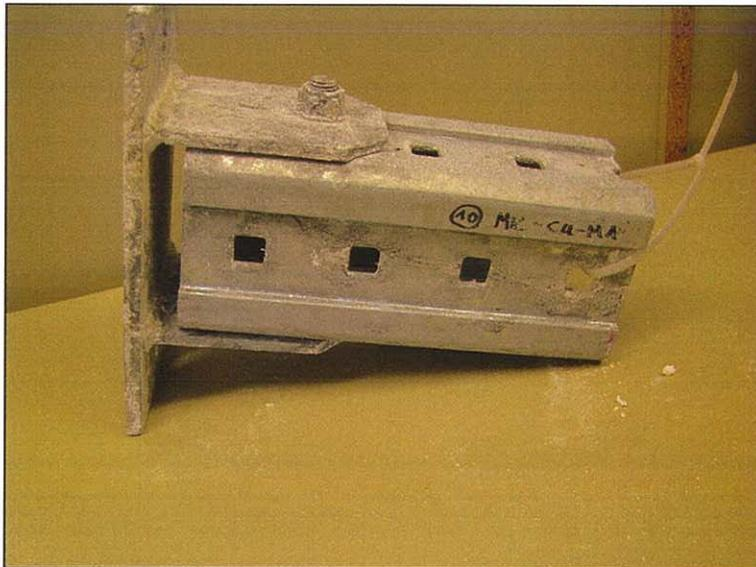
Pic. 21: Test object 10 after corrosion resisting conditioning
