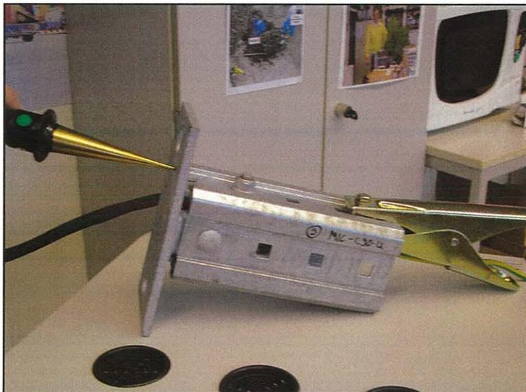
**Pic. 4:** Measuring setup before corrosion resisting conditioning
