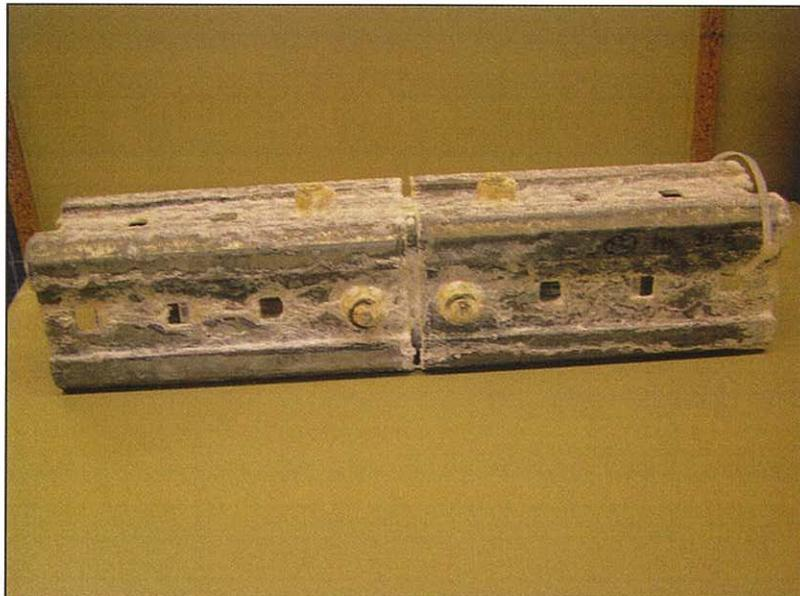
Pic. 22: Test object 12 after corrosion resisting conditioning
